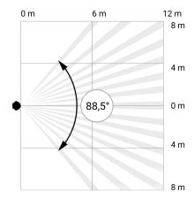
If the detector is not installed at the recommended height, this will reduce the area of the motion detection zone and impair the operation of the function of ignoring animals.
